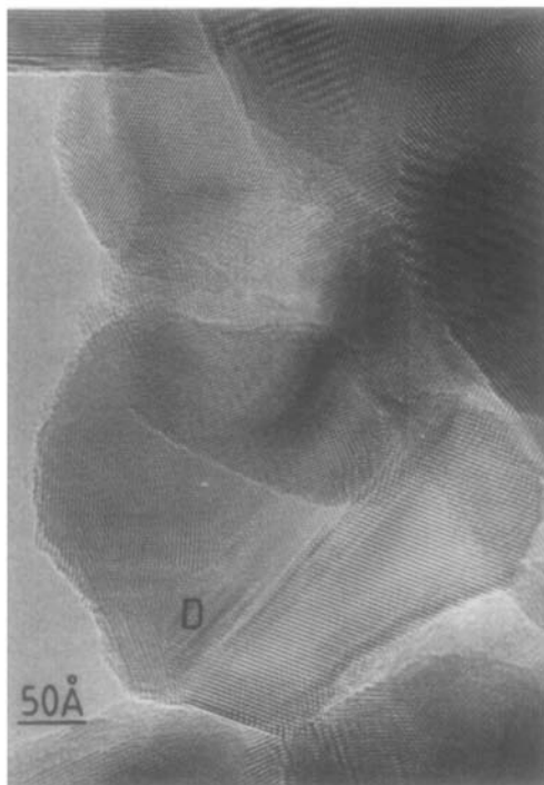
FIG. 2. Tin-molybdenum oxide B. High-resolution image showing typical particle morphology. The SnO 2 particle at D shows a well-ordered region separated from a highly distorted area by a twin boundary.
